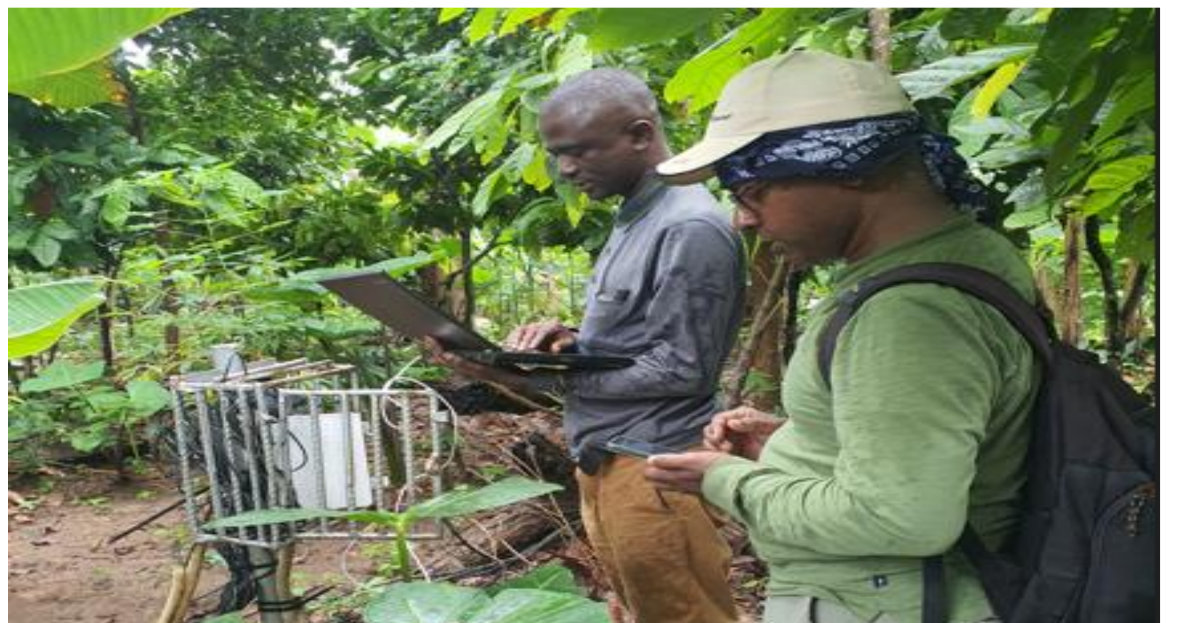
Plate 6. Soil sensors installed in a cocoa-agroforestry farm to collect data on soil physico-chemical properties (pH, moisture, electrical conductivity, etc.)
