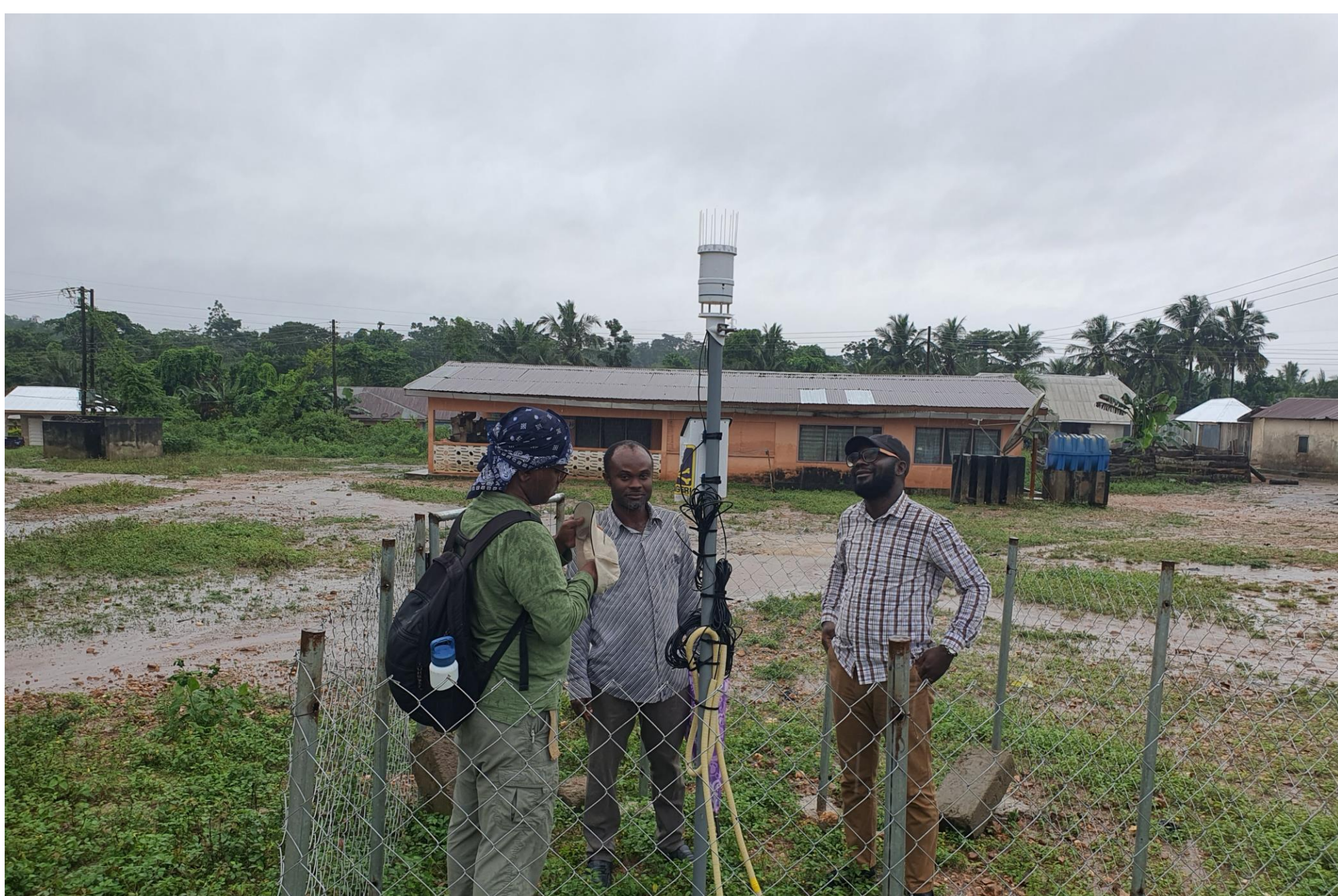
Plate 4. Automatic weather station for collecting data on different climatic conditions.
